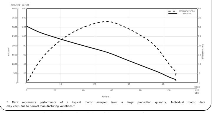
Data shown is measured at regulated nominal voltage and normalized to standard atmospheric pressure and temperature.
